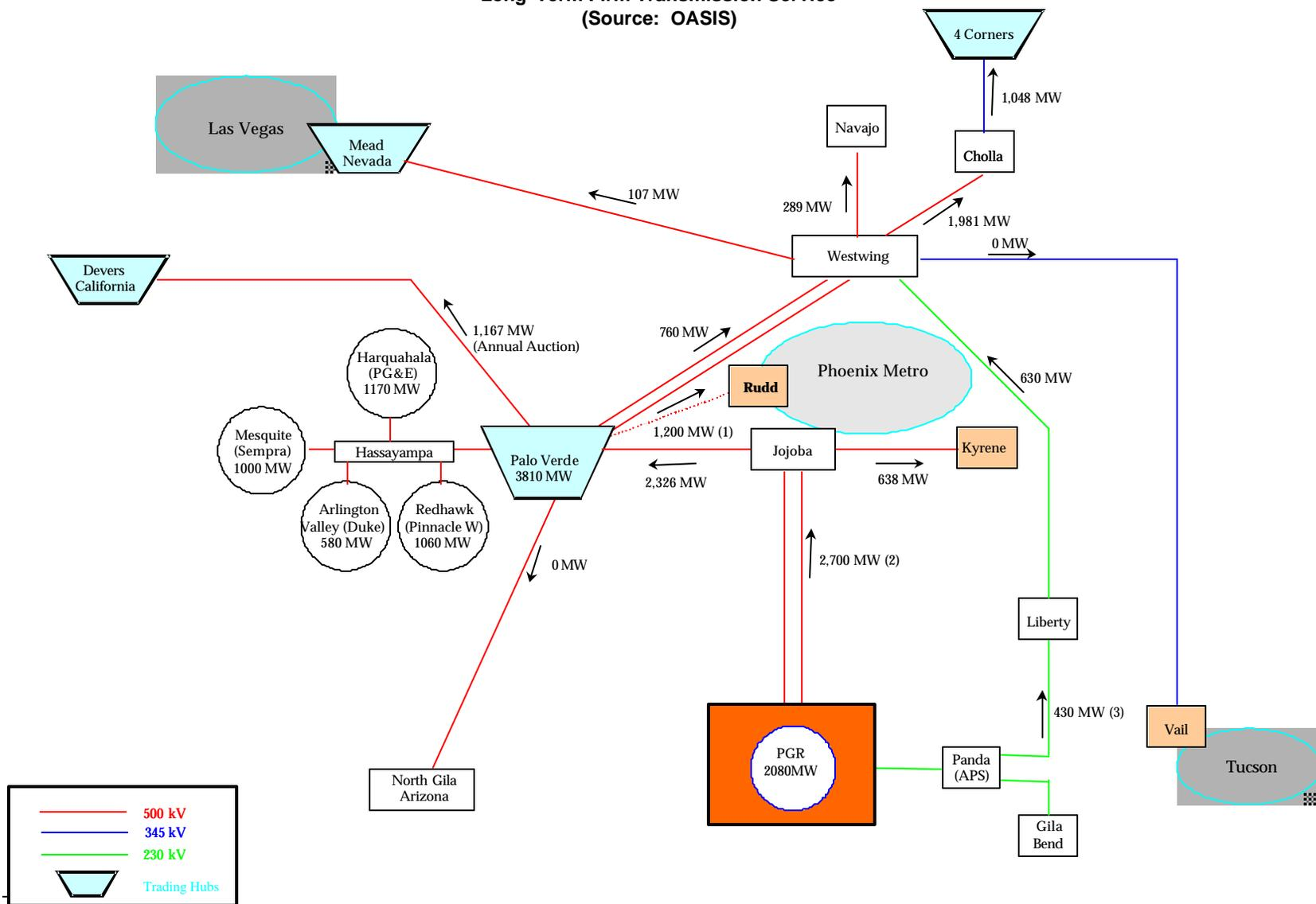
(1) Line under construction. The total expected line capacity will be 1,200, however, available firm transmission on this line not currently posted.
