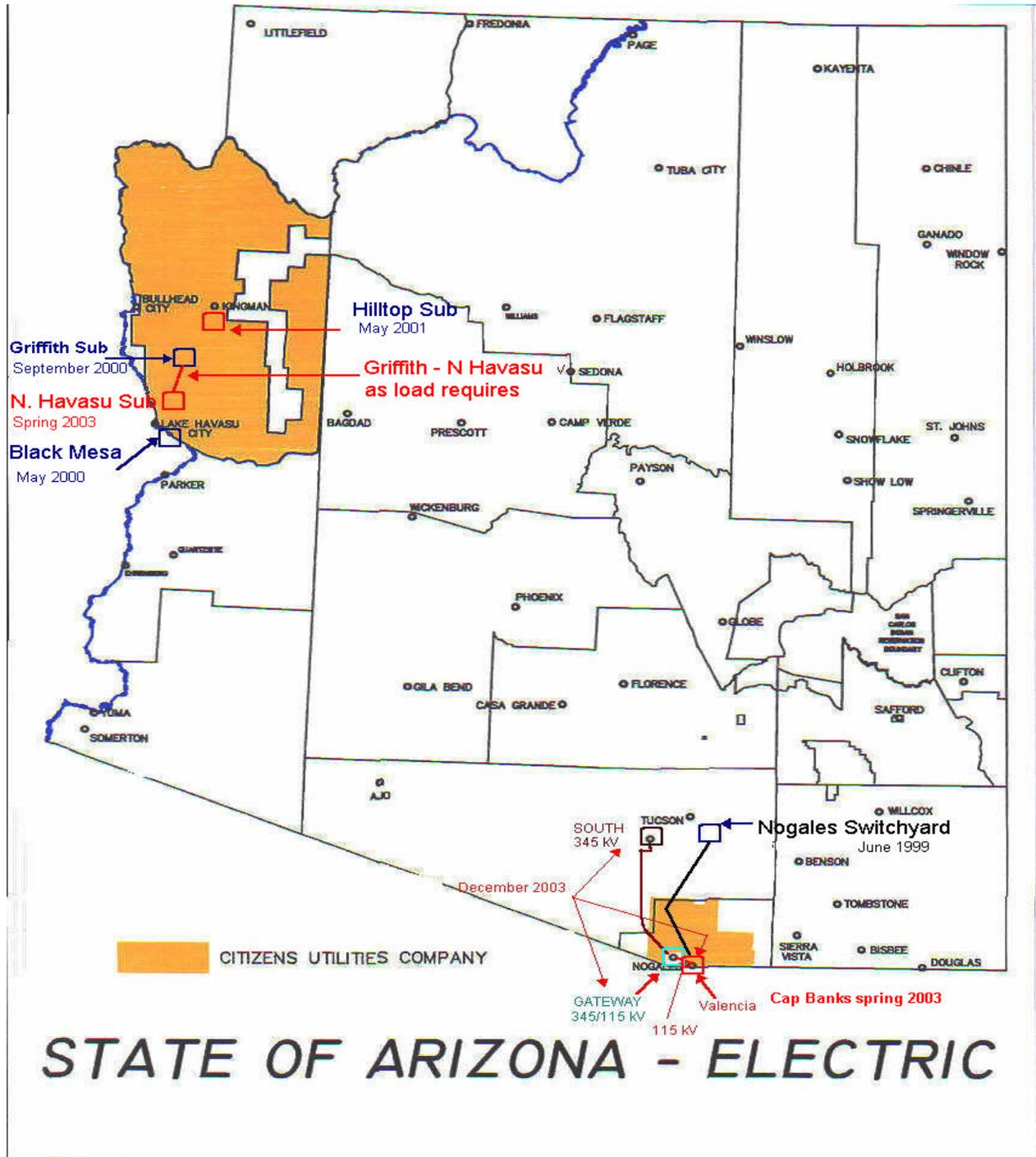
carry load, Citizens separates the load carried on the Valencia generation from the remainder of the system until the problem on the transmission line is repaired. In this case, that part of the load is isolated on local generation.
