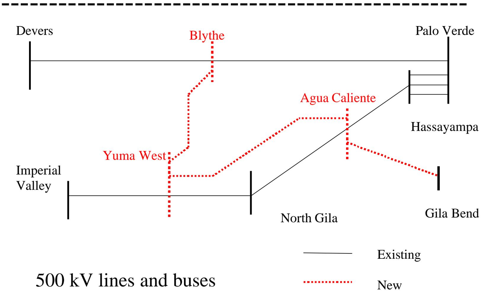
The NRG proposes a 500/230 kV project that could add 1,400 MW of transfer capability from the PV/Gila Bend area to the Southern California area. The NRG proposed project consists of the following elements depicted in Figure 6.6.
