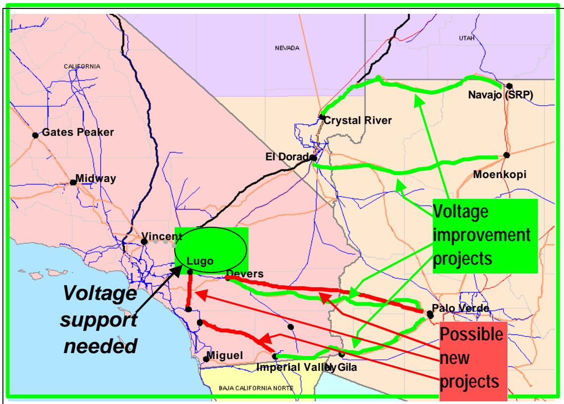
The STEP team identified a number of actions that could be taken to increase the transfer capability of the transmission in short-term. They have advanced these projects as first steps to increase transmission capability. The short-term upgrades are shown in green on Figure 11. They include:
