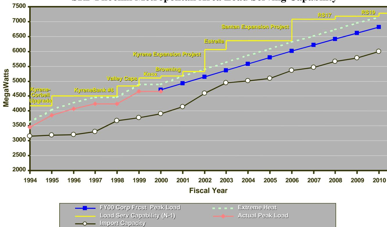
Without the Palo Verde to Southwest Valley 500 kV line in 2003, APS peak load serving capability would be inadequate until construction of the Trilby Wash to El Sol 230 kV line in 2006. Similarly, without the Palo Verde to Southwest Valley 500 kV line in 2003 and the 575 MW reduction of the Kyrene plant expansion in 2002, SRP’s load serving capability would be inadequate to meet its peak load obligations until the Santan plant expansion in 2006.
