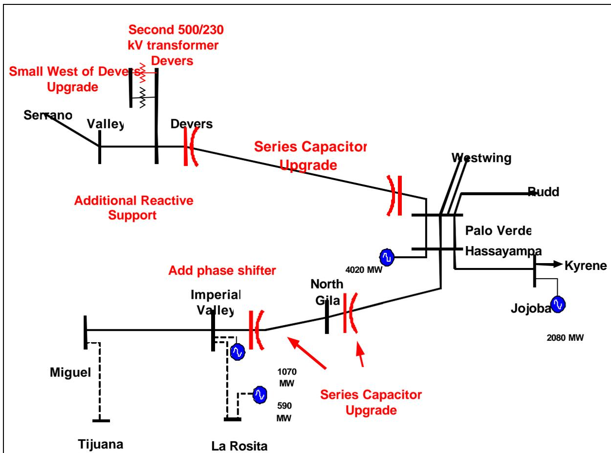
For the long-term, new transmission will have to be built to provide additional transmission capability across this Path. The transmission lines shown in red on Figure 11 are the most-likely additions. The first new addition is a second Palo Verde – Devers 500 kV transmission line into the Los Angeles area. The other new project would add a 500 kV transmission line from Imperial Valley to Lugo through the edge of San Diego.
